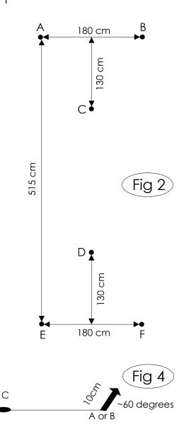
Pegs at A and B angled AWAY from C Pegs at E and F angled AWAY from D
